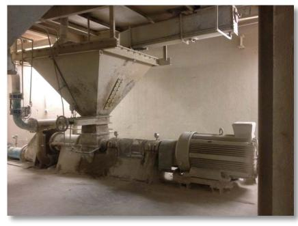
Figure 3: The old screw pump
