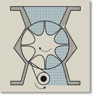
Figure 2: Mode of operation of a self-cleaning rotary valve
