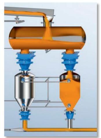
Figure 6: Interconnection of several pressure vessels for quasicontinuous conveying
