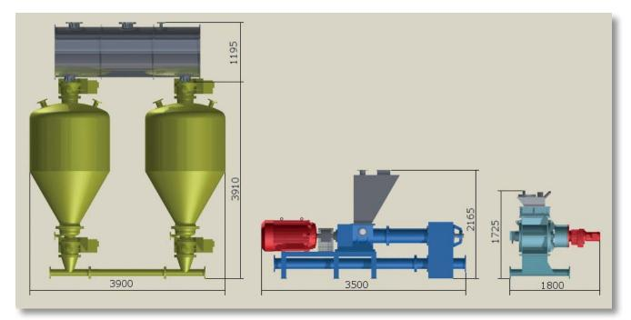
Figure 8: Comparison of the geometries of a pressure vessel system, a screw pump and a rotary valve using the example of cement conveying [1] at a conveying rate of 50 t/h
