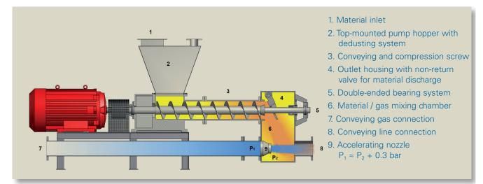
Figure 5: Functioning principle of a screw pump [1]
