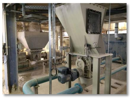
Figure 1: Metering and conveying system from Kreisel
