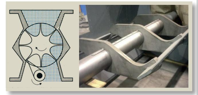
Figure 10: a) Functional principle of a self-cleaning rotary valve, b) Scraper wheel in dismantled condition
