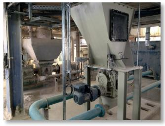
Figure 11: Self-cleaning rotary valve for pneumatic conveying of bypass dust at the cement works Karsdorf of Opterra
