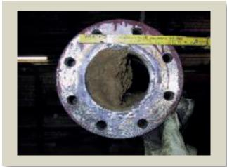
Figure 4: Bonded delivery pipe [5]
