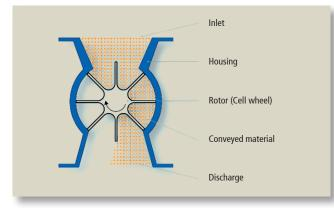
Figure 7: Functional principle of a rotary valve
