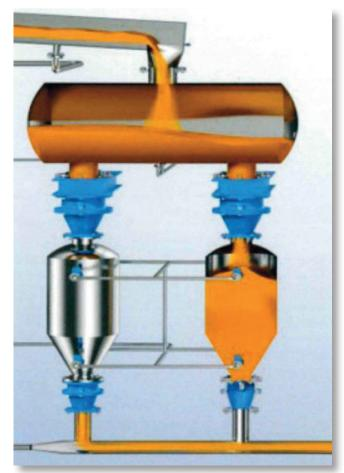
Figure 5: Interconnected pressure vessel system
