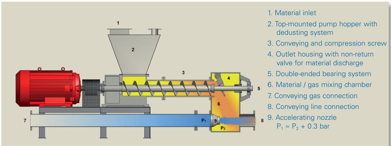
Figure 5: Functioning principle of a screw pump [1]
