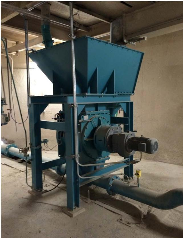
Figure 4: The new Kreisel rotary valve
