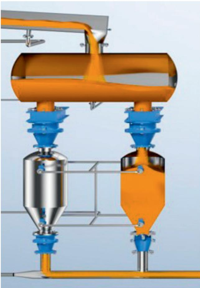
Figure 6: Interconnection of several pressure vessels for quasi-continuous conveying
