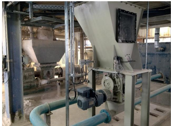
Figure 11: Self-cleaning rotary valve for pneumatic conveying of bypass dust at the cement works Karsdorf of Opterra
