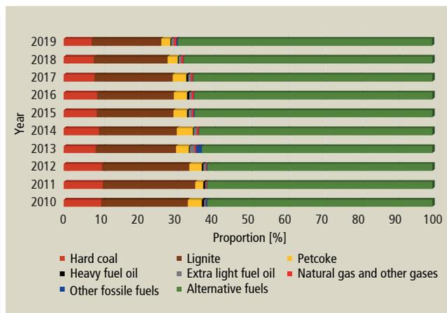
Figure 2: Fuel energy use by energy source from 2010 to 2019 [3] in %
