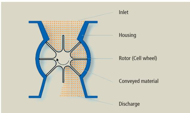
Figure 7: Functional principle of a rotary valve
