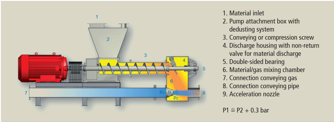
Figure 6: Core components of a screw pump
