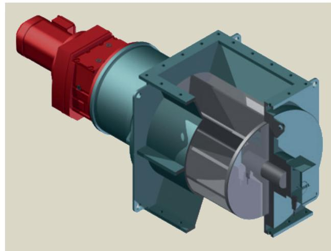
Figure 8: The Kreisel rotary valve in spatial representation
