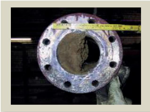
Figure 4: Bonded delivery pipe [5]
