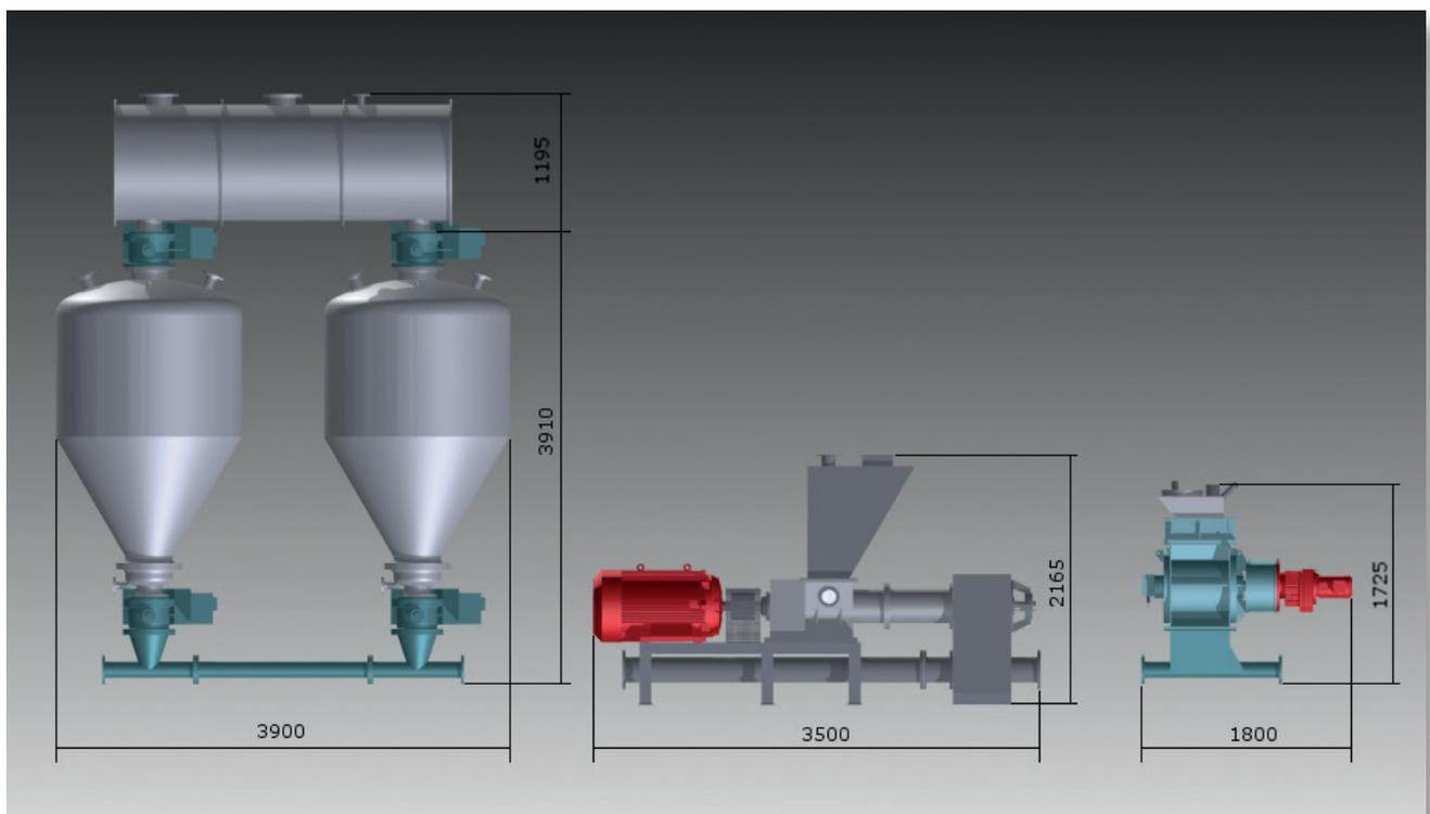
Figure 9: Size comparison of the three injection systems
